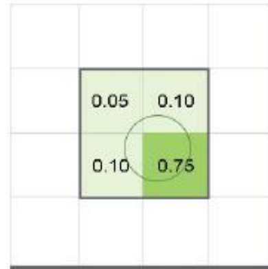
Charge collects in each pixel.
