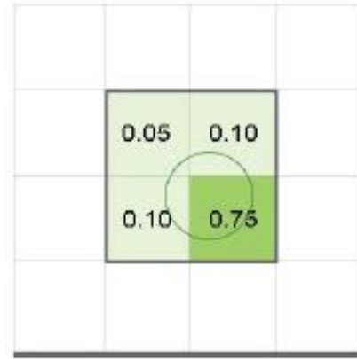
Charge collects in each pixel.
