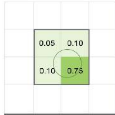
Charge collects in each pixel.
